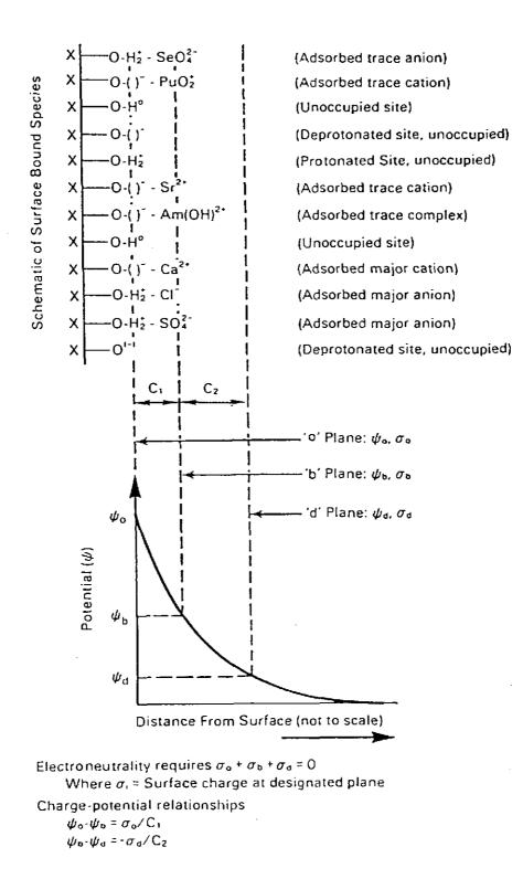
Figure 1. Schematic Representation of Triple Layer Adsorption Model.
